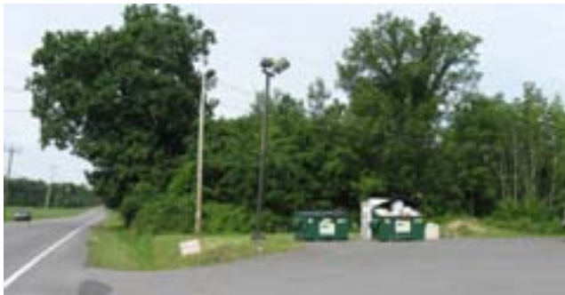
Proper siting of utilitarian functions on a site are essential. It would be preferable to locate this trash area at a back corner of the parking lot and screen it with a trash enclosure.
