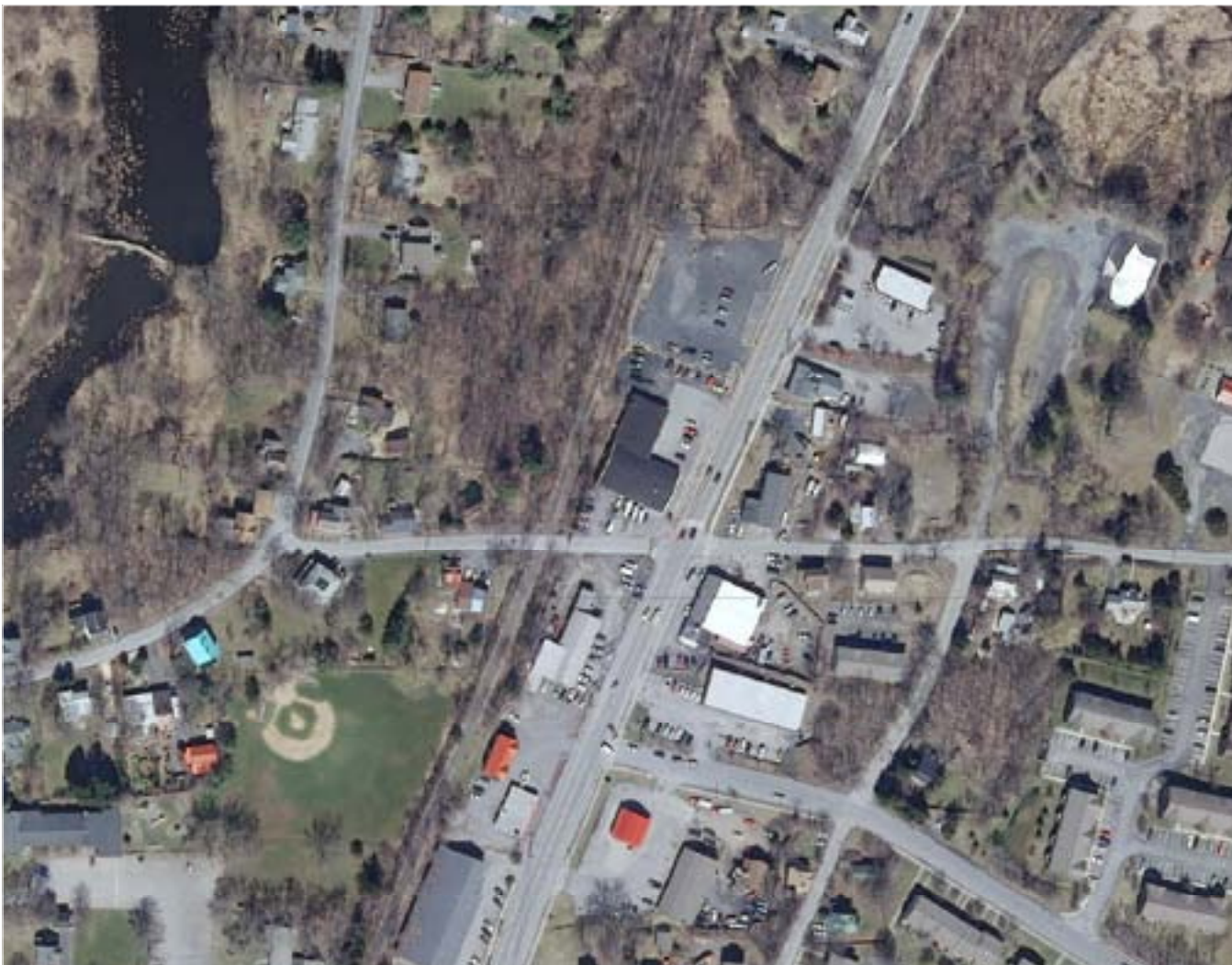
Extensive parking, uncoordinated curb cuts, little landscaping, and varied building footprints and front-ages are typical of commercial highway development in the Shawangunk region. This area is along Route 32 north of New Paltz Village.
